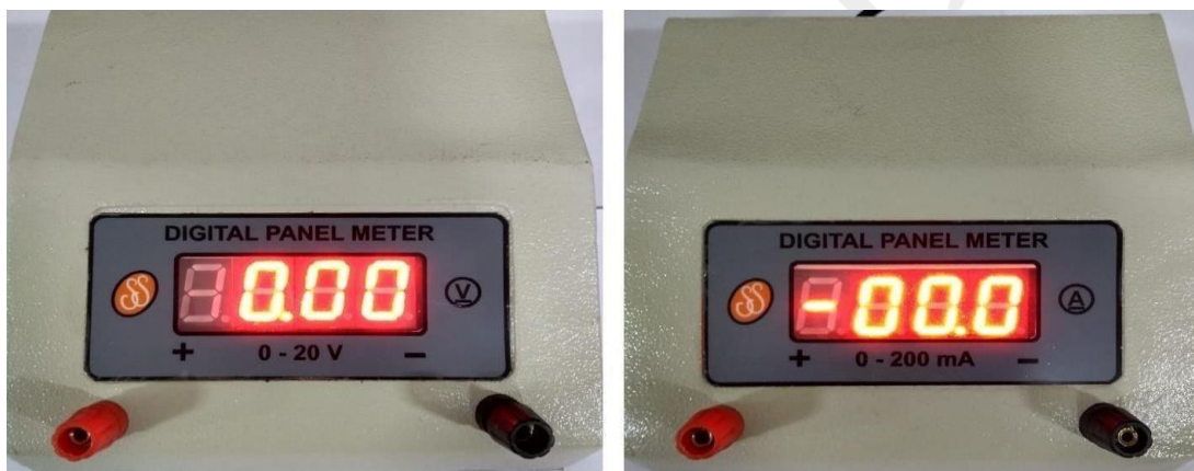
Fig.7: Digital Voltmeter and Ammeter
